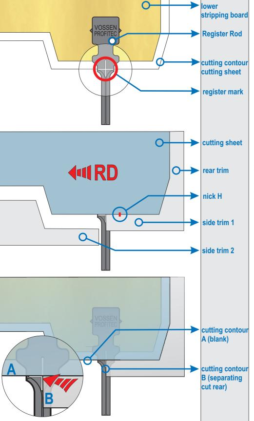
Register Rod is a further development of the proven Strip Rod for separating of trim waste. The Register Rod has a register mark. Herewith the exact positioning of the lower stripping board can be
